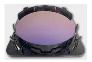
Silicon wafer deposited oxide layer due to its excellent dielectric properties which is widely applied in semiconductor industry. Thermal Oxide is typically grown in a diffusion furnace (either vertical or horizontal one) and is grown at high temperatures from 800°C to 1200°C via either a "Wet" or "Dry" growth technique. USIC provides high quality thermal oxide wafers especially in diameter of 200mm and 300mm.
